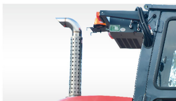
Equipped with high exhaust as standard, which is humanized design, anti water spray and thermal insulation.
