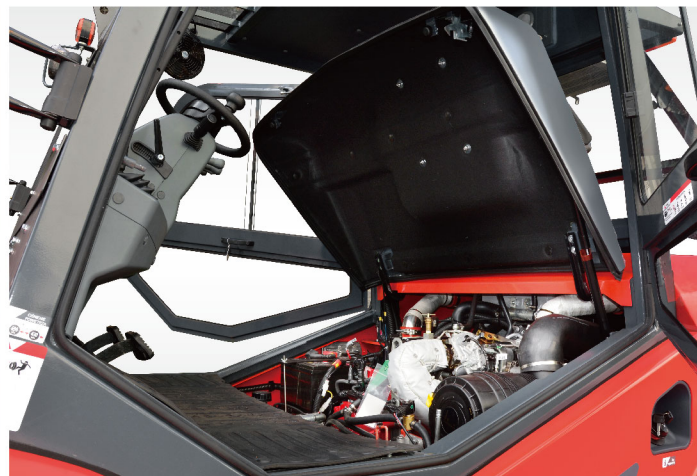
The hood has a large opening angle, greatly improving maintenance space.
