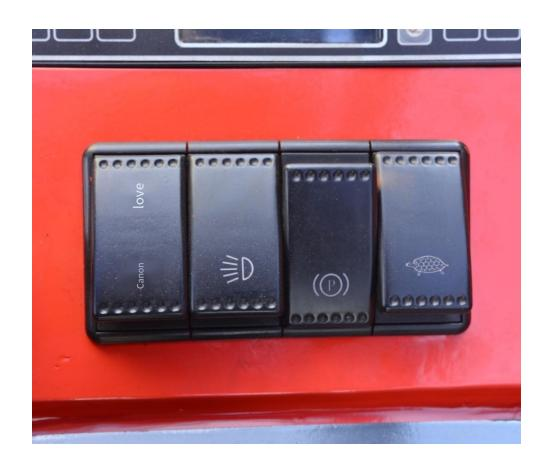
■ High and low speed switch. Select high speed driving mode when using rear wheel drive. Select low speed driving mode when using full wheel drive. One key switch for high
