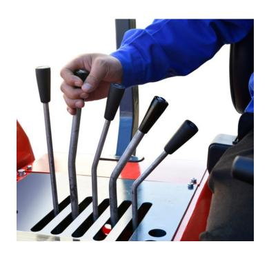
■ The standard five-piece valve is equipped with compound, which can realize seven functions, such as lifting of the mast, extending and retracting of the mast, extending and retracting of the cargo fork, tilting, lateral movement of the mast, pressing and opening of the press plate, and extending and retracting of the leg
